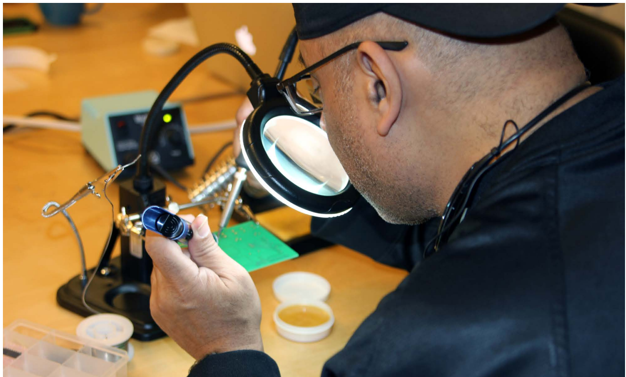
A BCDI trainee practices soldering electronic components to a circuit board.
